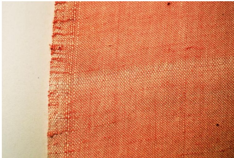
Figure 1: Selvedge on hand-woven cloth sample produced at Thanapara. The selvedge (edges) of handwoven cloth are often indicators of a weaver's skill level as it is tacit knowledge – controlled by 'feel' and learned through experience (Yarwood 2020)
