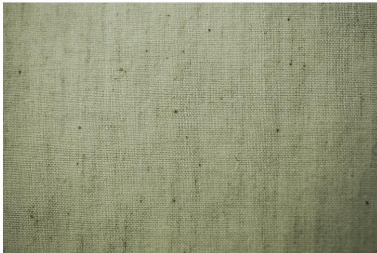
Figure 6: Specks of ‘dust’ stuck in woven cotton cloth produced for Bhalo by Thanapara. This cloth was rejected by another buyer (Yarwood 2020)
